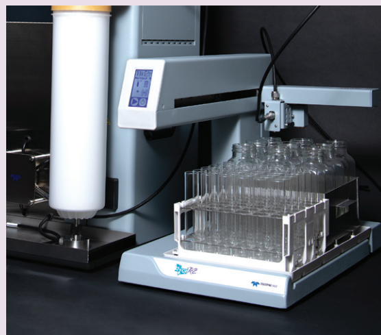
Foxy ® R2 Daisy-chain up to four Foxy R2 fraction collectors for hundreds of fractions. Choose from a variety of collection containers.
