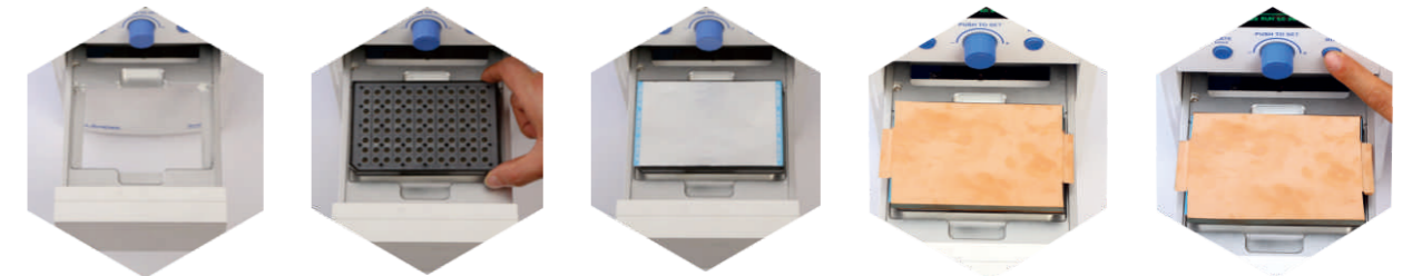
Step.1 Pull the drawer Step.2 Put the adapter plate Step.3-1 Put a sealing film Step.3-2 Put the weighted seal platen if the film is curly Step.4 Press "RUN"
