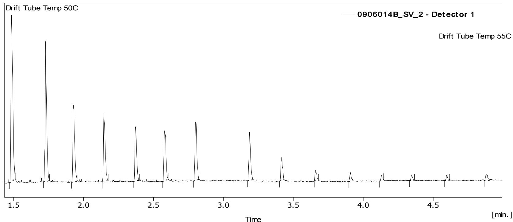
This example show that a small increase in drift tube temperature will decrease the signal of the analyte significantly.
